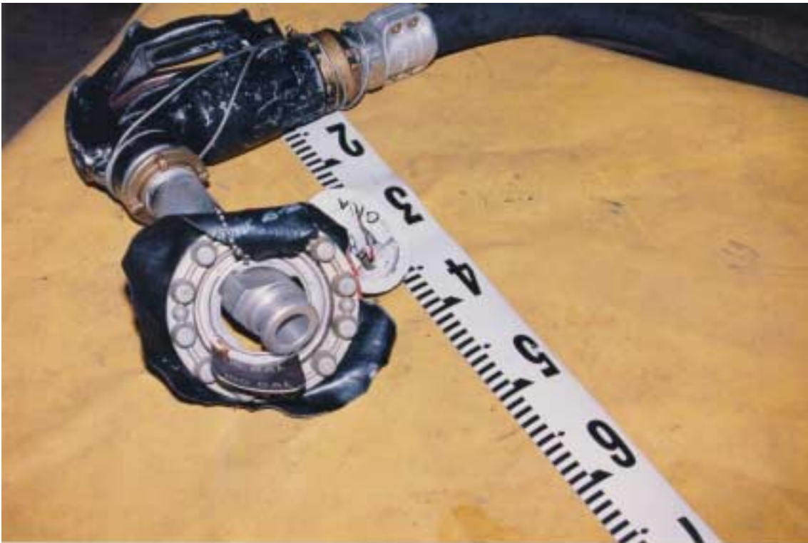
Fitting of the Camlock coupling into the reduced orifices intended for aviation gasoline
