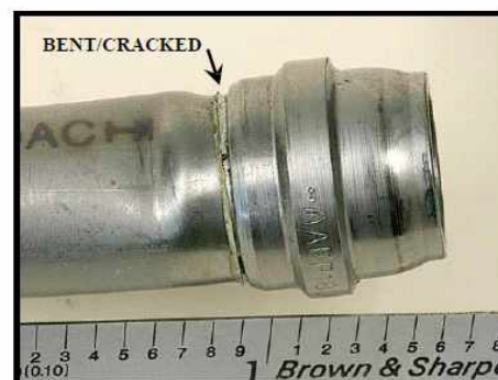
Figure 5. Detailed view of Return Lines from Left CLG Anti-Skid Manifold (C-1)- Bent and Cracked End Fitting.
