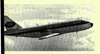
accordingly limited to a maximum indicated airspeed of 140kt and an altitude of 3,000ft. Flight tests were pushed out towards the edges of the envelope: 330kt IAS, Mach 0.74 diving speed; 285kt IAS, Mach  $0.65 V_{MO}$ . Real-time data monitoring and transmission was used to assist in observing the flights.
