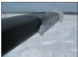
**Photo 4.** Ice on the horizontal stabilizer leading edge
