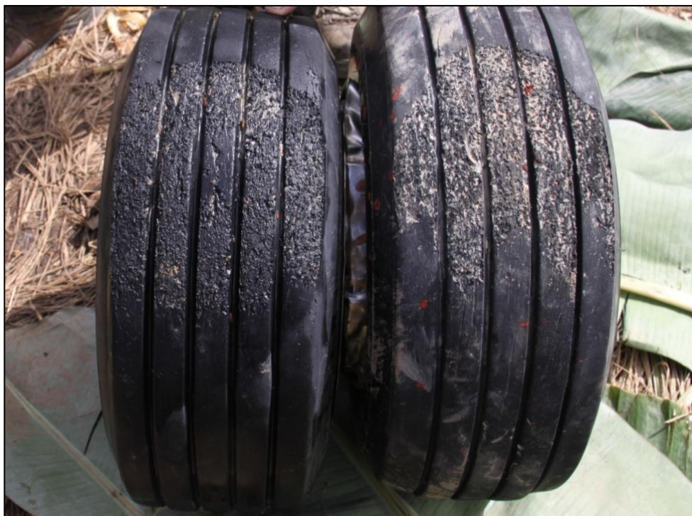
Figure 9: Abrasion damage to the left and right main landing gear tyres
