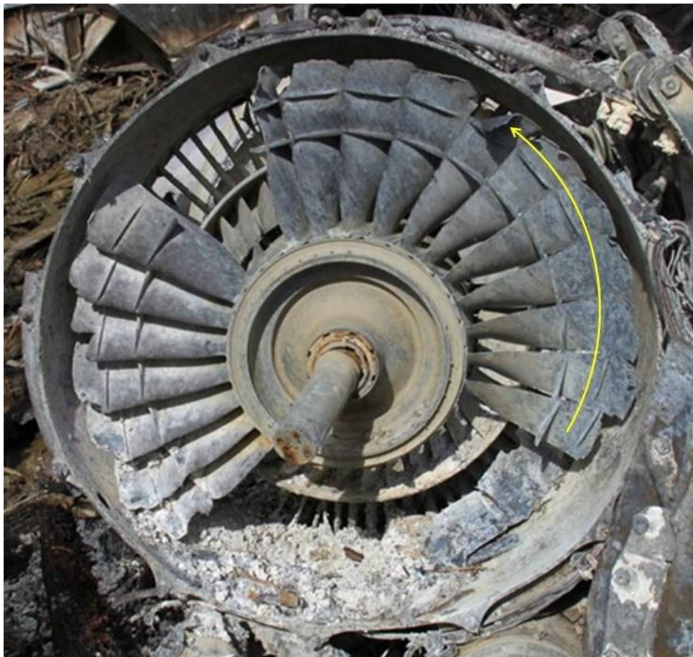
Figure 8: Right engine showing indications of rotational damage
