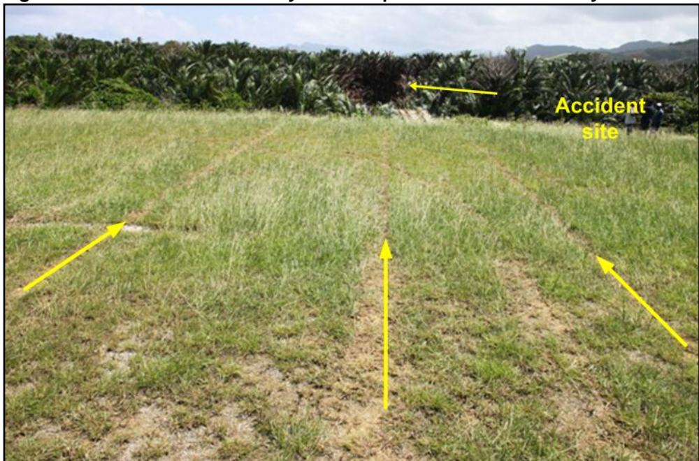
Figure 11: Wheel track marks beyond the upwind end of the runway
