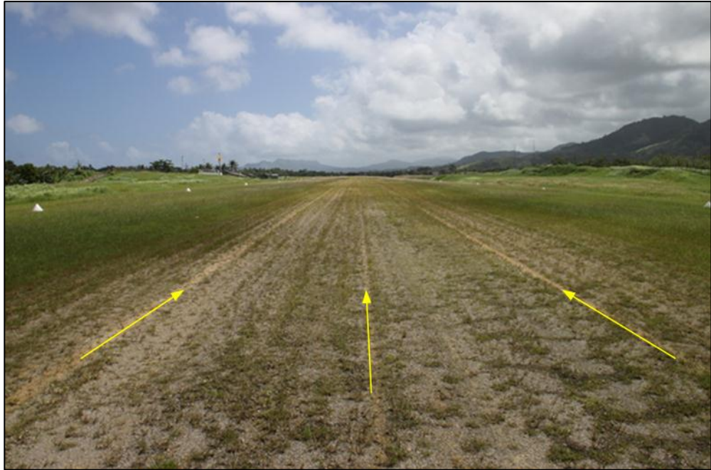
Figure 11: Wheel track marks beyond the upwind end of the runway
