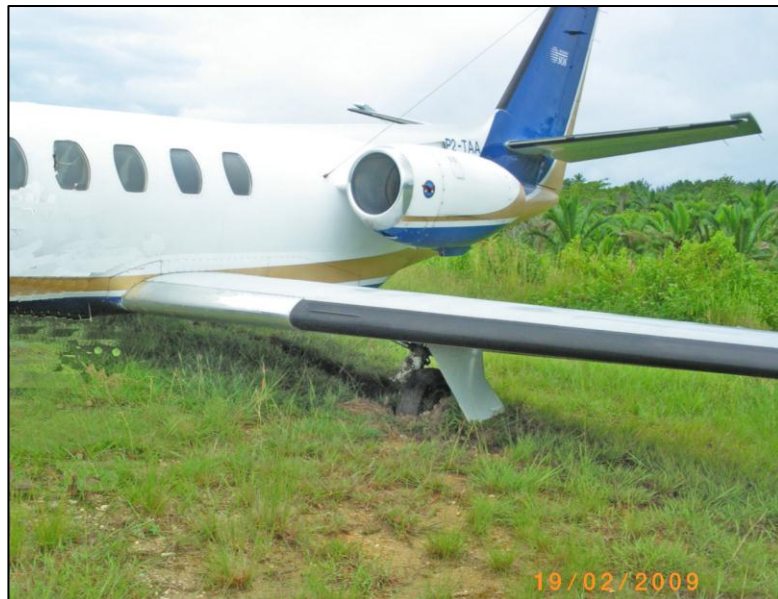
Figure 17: Left main landing gear bogged
