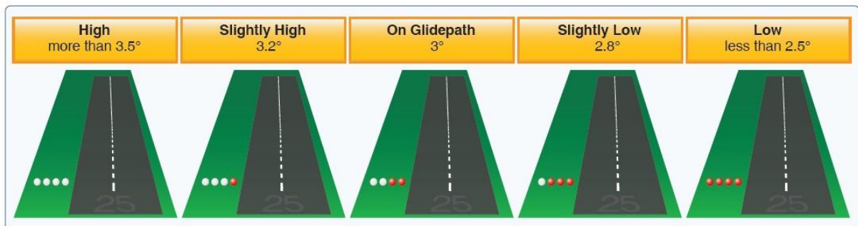
Fig. 2: PAPI indications of different approach angles
