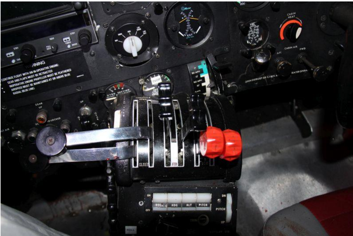
Fig. 12: Twisted centre quadrant including engine control levers
