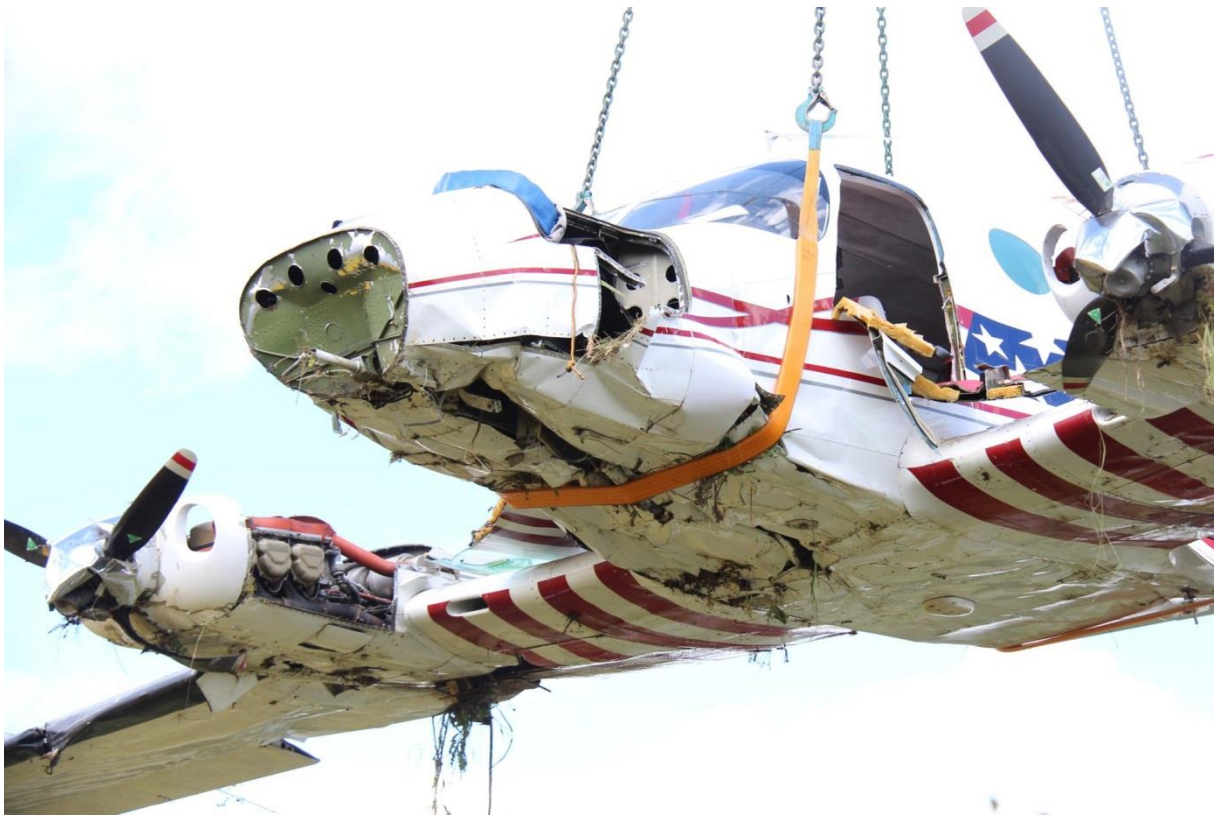
Fig. 11: Damage at the front of the fuselage
