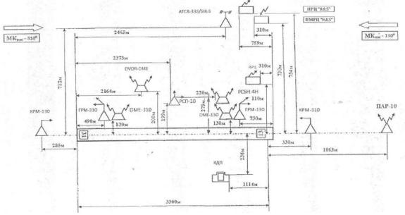
Fig. 5. Layout of radio equipment of the Lviv aerodrome relative to the runway
