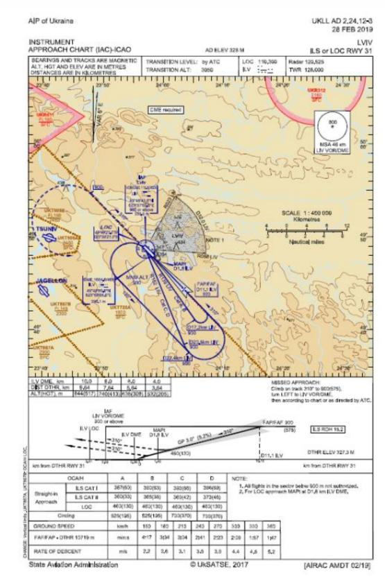
Fig. 6. Excerpt from the Aeronautical Information Publication of Ukraine (RW-31 instrument approach procedure)
