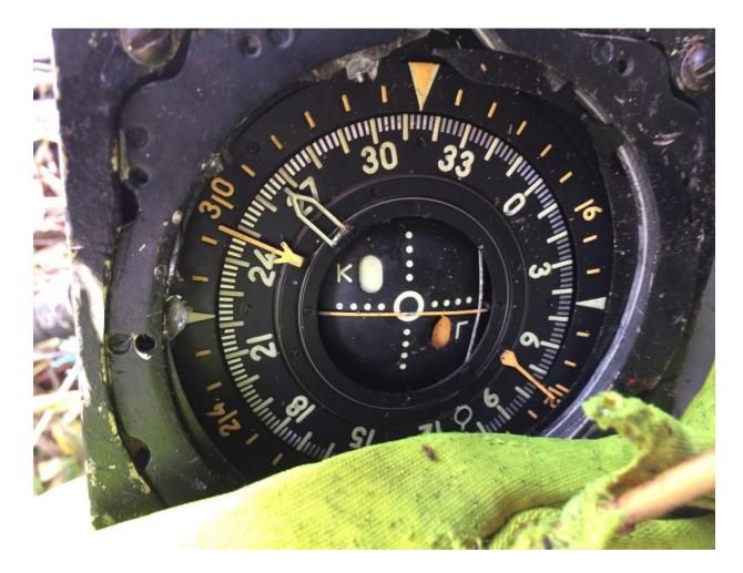
Fig.7 Pointer of the flight control and navigation instrument
