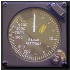
Fig. 4 Radio altimeter indicator
