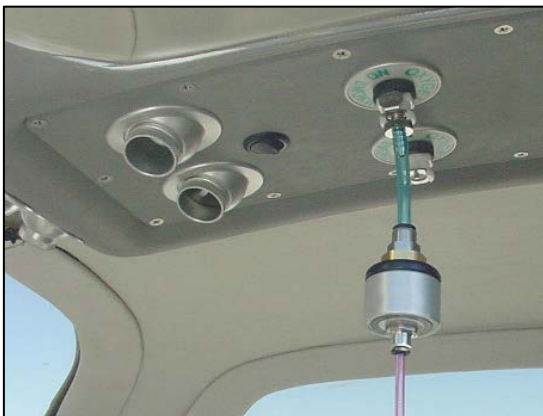
Figure 7: In-line regulator to connect EDS to aircraft oxygen outlet
