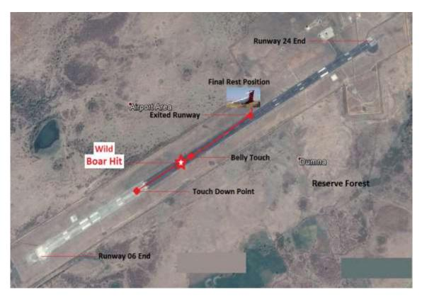
As per the evidences collected at the accident site, the aircraft made touch down at a distance of 595 meters from the runway 06 end. After about 254 meters of landing roll the left main landing gear of the aircraft hit the wild boars on runway. Due impact with the boars the left main landing gear collapsed. Continuous marks of propeller blade strike were observed on the
