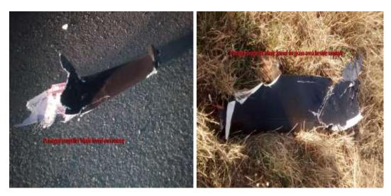
Damaged Propeller on the runway and shoulder area
