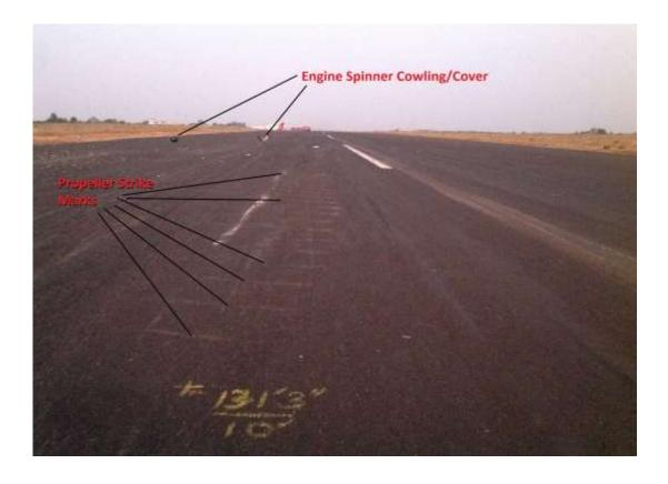
Subsequently the aircraft belly came in contact with the runway surface and belly scraping marks were observed on runway for about 168 meters. All the five propeller blades were sheared off from the root attachment. The damaged propeller blades were found on runway and on the basic strip.
