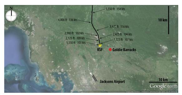
Figure 2: Final part of the track taken by KSF; the dotted white arrow shows the approximate path to be flown from a left base position onto runway 14 right
