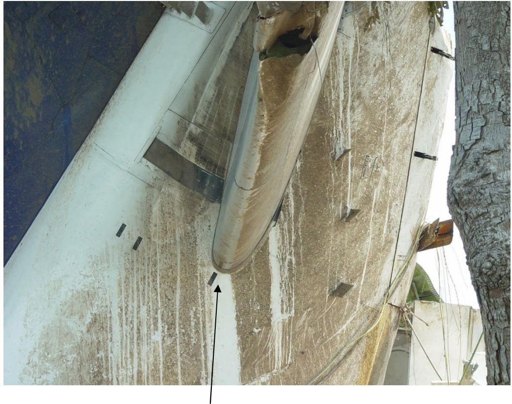
Fig 4-4 Tail part of the aircraft showing horizontal stabilizer in the full nose up pitch altitude
