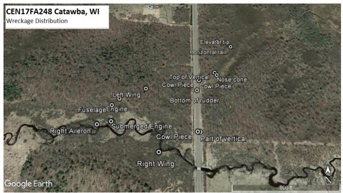
Figure 1. Wreckage Distribution
